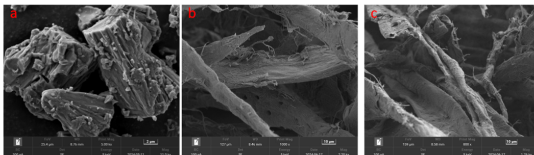
FIGURE 10 SEM images. (a) Pure dye; (b) Pristine pulp fibers; (c) Pulp fibers after dyeing.
